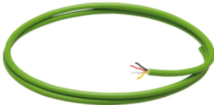
**GEWISS KNX BUS CABLES - LSZH CABLE SHEATH - 4 CONDUCTORS 2 X 2 X 0,8 - DIAMETER 6,1MM - GREEN**
